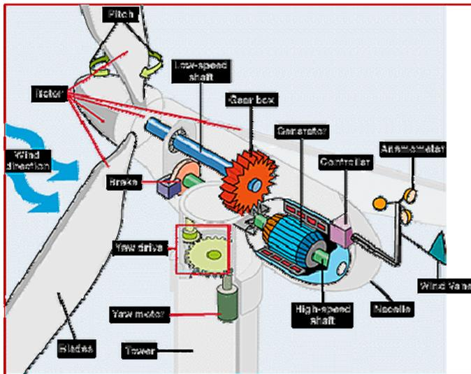
Fig. 1 The components of a common horizontal-axis turbine
