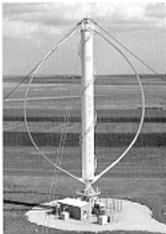
Fig. 4 Vertical-axis turbine (Darrieus design)
